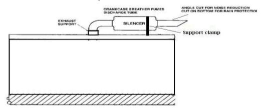
The silencer and the exhaust system should be complied as per the specifications and picture shown above.
