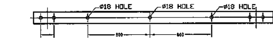
GI SWITCH SUPPORTS FOR ABS, 2 NOS.
