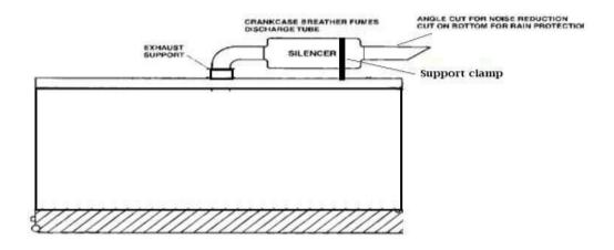
The silencer and the exhaust system should be complied as per the specifications and picture shown above.
